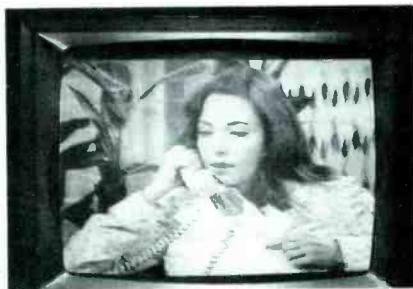
Fig. 9 A small picture, both vertically and horizontally, results from an open C213, or a line voltage of only about 70 volts RMS.
