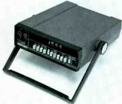
The Fluke 8000A 3 1/2 digit multimeter
