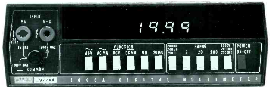
Resolution is 100 microvolts, 100 nanoamps and 100 milliohms
