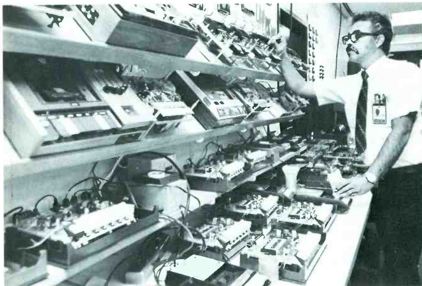
Fig. 1 Random samples of cassettes from current Memorex production are tested for performance and durability on many brands of machines.
